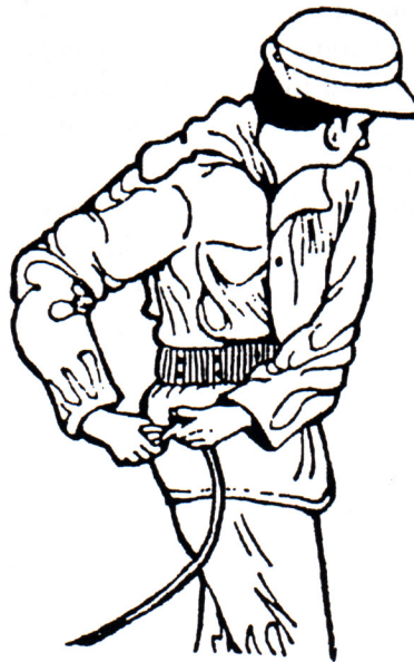
Holding the fuse while crimping.
